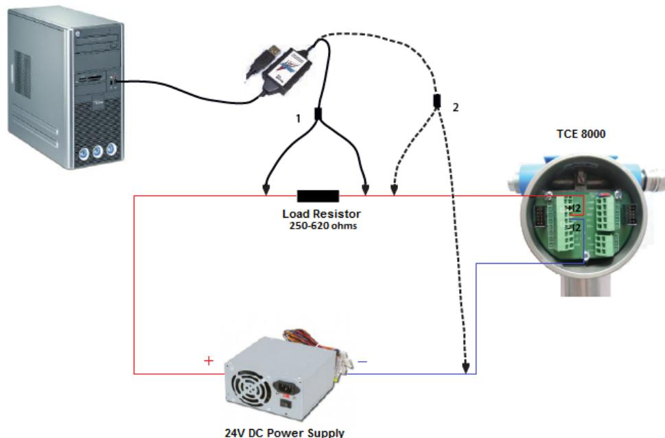
Connect the test clips of the HART® modem across the load resistor (1). If in a fixed installation a load resistor of the required size is built in, but not accessible, a HART® modem without built in load resistor can be connected across the TCE 8000 (2).
