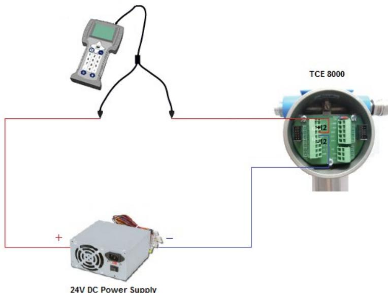
Connect the clip of the Field Communicator to the bare end of the wires.
