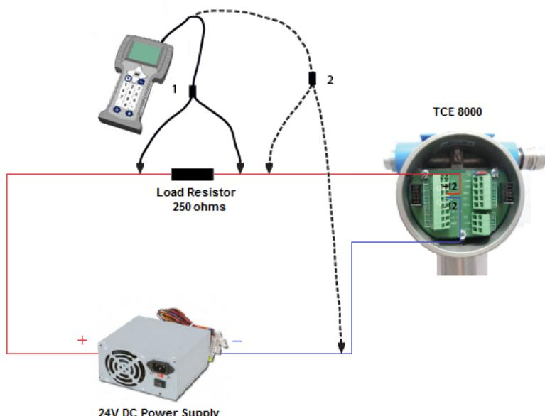
Connect the test clips of the Field Communicator across the load resistor (1).
