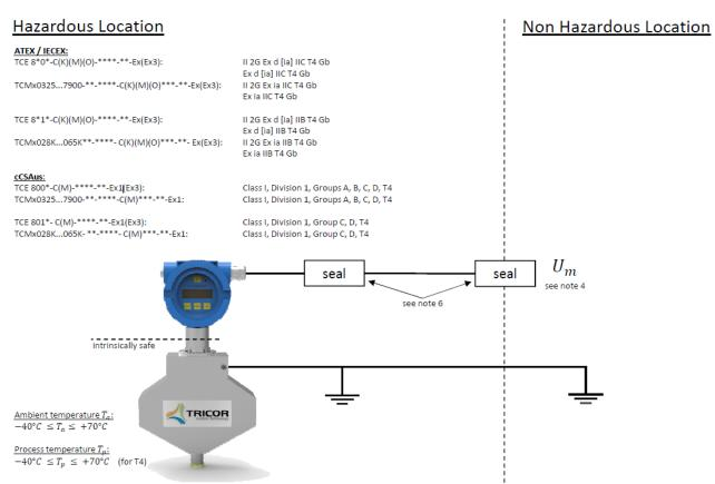
Housing of Transmitter and Sensor shall always be connected as illustrated
