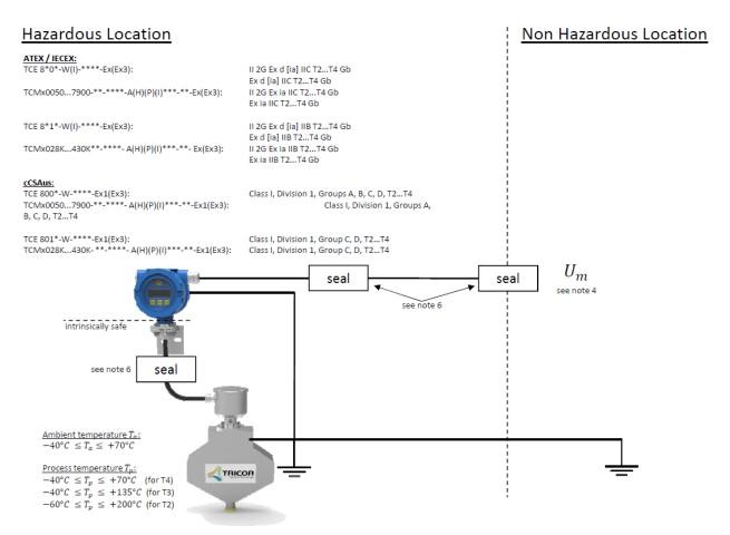
Housing of Transmitter and Sensor shall always be connected as illustrated
