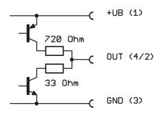
The output drivers are asymmetrical push pull output stages with the protective resistors of 720  $\Omega$  and 33  $\Omega$  as shown.
