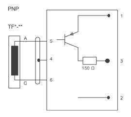
To connect the amplifier, shielded cables must be used. The shield should be connected to the case. For operation in hazardous areas a good connection of PE is mandatory. Therefore please apply the signal cable shield either to the cable gland of the amplifier or to the grounding screw (see drawing below).
