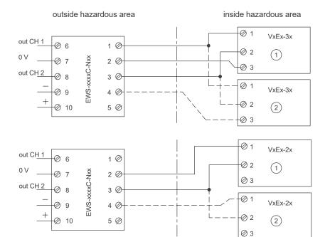
EWS = intrinsically safe power supply and separation amplifier
